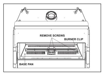
Figure 16.4 Remove Burner Assembly
